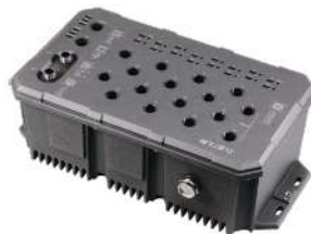
LMX-1600G-M12-67-110(-T) 16-Port Industrial M12 IP67 Waterproof Gigabit Light Layer 3 Managed Ethernet Switch, with 16*10/100/1000Tx M12 Connectors (X-Coded); 24~110VDC Power Input
