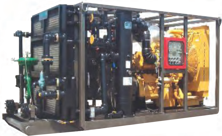
Diesel Powered Nitrogen Gas Booster with capacity from 300 - 1,000 SCFM (510 m 3 /hr) and outlet pressures from 350 - 5,000 PSIG (24 - 345 BARG)
