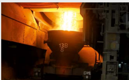
Monitoring of the refractory lining of a slag ladle car while pulling out of the factory
