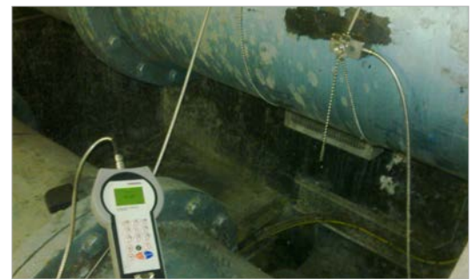
KATflow 200 installed on large sewage pipe
